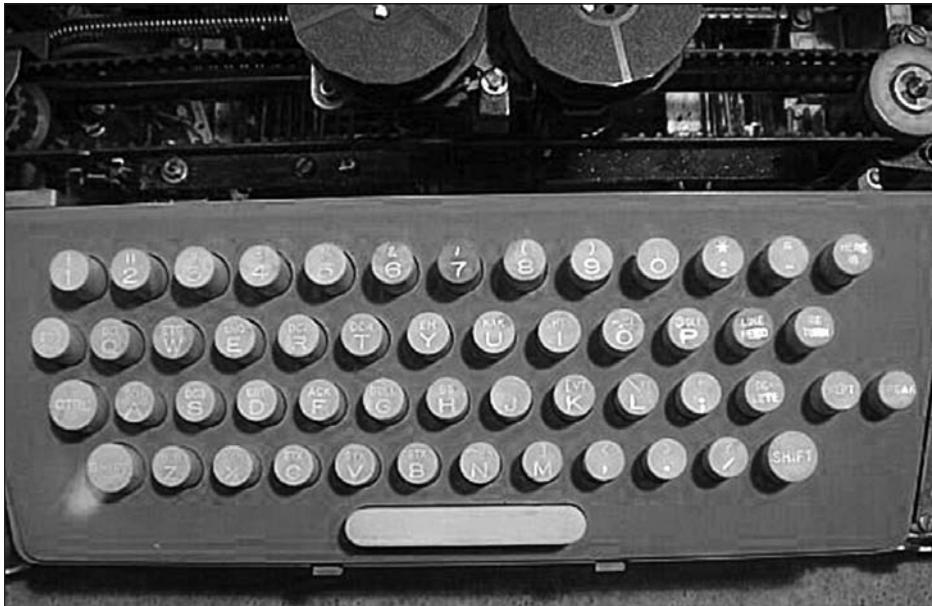
**FIGURE 4-1:** Keyboard of the Teletype ASR33
