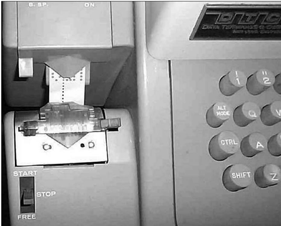
**FIGURE 3-3:** Close-up of a Teletype 33-ASR
