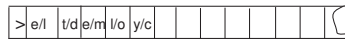
Figure 1.5 To simulate a machine M with alphabet \Gamma that has tapes infinite in both directions, we use a machine \tilde{M} with alphabet \Gamma^2 whose tapes encode the “folded” version of M 's tapes.
