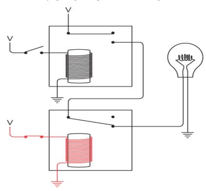
The lightbulb is still not lit. The current can't reach the lightbulb because the first relay isn't triggered. The only way to get the bulb to light up is to close both switches:
