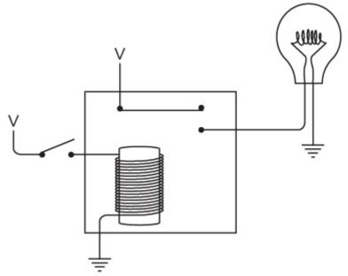
When the switch is closed, the bulb lights up.
