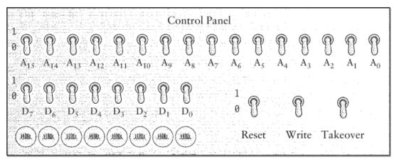
Unlike the earlier control panel, this one has a switch labeled Reset. The Reset switch is connected to the Reset input of the microprocessor. As long as that switch is on, the microprocessor doesn't do anything. When you turn off the switch, the microprocessor begins executing machine code.
