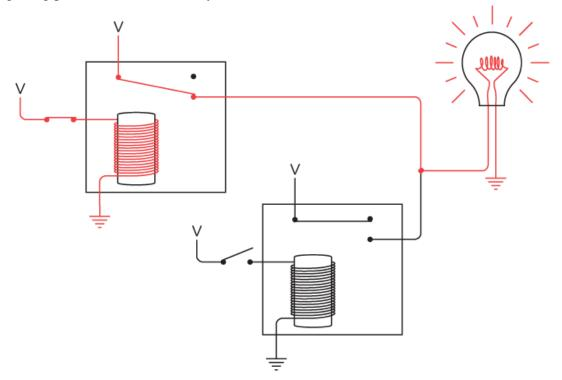
Similarly, if we leave the top switch open but close the bottom switch, the bulb lights up:
