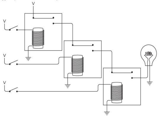
The lightbulb lights up only if all three switches are closed. This configuration is expressed by this symbol:
