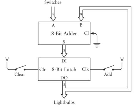
As you'll recall, an 8-bit latch uses flip-flops to store an 8-bit value. To use this device, you first momentarily press the Clear switch to set the stored contents of the latch to all zeros. Then you use the switches to enter your first number. The adder simply adds
