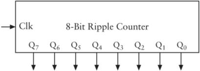
This is called a *ripple* counter because the output of each flip-flop becomes the Clock input of the next flip-flop. Changes ripple through the stages sequentially, and the flip-flops at the end might be delayed a little in changing. More sophisticated counters are *synchronous*, in which all the outputs change at the same time.
