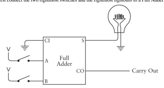
When you begin adding two binary numbers, the first column of digits that you add is different. It's different because every subsequent column might include a carry bit from the previous column. The first column doesn't include a carry bit, which is why the carry input to the Full Adder is connected to ground. That means a 0 bit. The addition of the first pair of binary digits could, of course, *result* in a carry bit. That carry output is an input to the next column.
