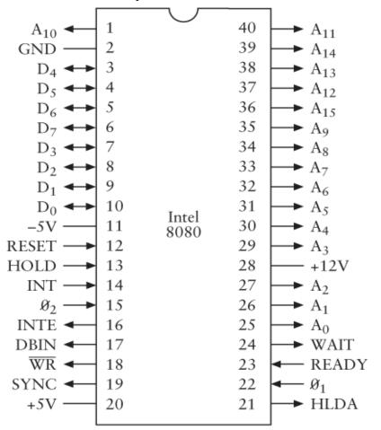
Every electrical or electronic device that we've built in this book has required some kind of electrical power supply. One of the 8080's quirks is that it requires *three* power supply voltages. Pin 20 must be connected to a 5-volt power supply, pin 11 to a -5-volt power supply, and pin 28 to a 12-volt power supply. You connect pin 2 to ground. (In 1976, Intel released the 8085 chip, which simplified these power requirements.)
