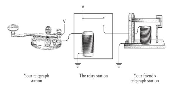
The relay is a remarkable device. It's a switch, surely, but a switch that's turned on and off not by human hands but by a current. You could do amazing things with such devices. You could actually assemble much of a computer with them.
