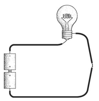
The two positive ends of the battery need electrons for the chemical reactions, but there's no way electrons can get to them because they're attached to each other. If the two positive ends of the battery are connected, the two negative ends should be also:
