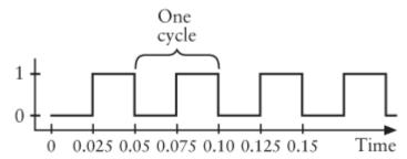
The *frequency* of the oscillator is 1 divided by the period. In this example, if the period of the oscillator is 0.05 second, the frequency of the oscillator is  $1 \div 0.05$ , or 20 *cycles per second*. Twenty times per second, the output of the oscillator changes and changes back.
