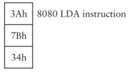
will load the accumulator with the byte stored at memory address 347Bh. Now compare that with the 6800 *LDA* instruction using the so-called 6800 extended addressing mode:
