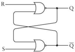
The output that we used for the lightbulb is traditionally called Q. In addition, there's a second output called  $\overline{Q}$  (pronounced *Q bar*) that's the opposite of Q. If Q is 0, then  $\overline{Q}$  is 1, and vice versa. The two inputs are called S for *set* and R for *reset*. You can think of these verbs as meaning "set Q to 1" and "reset Q to 0." When S is 1 (which
