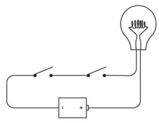
Switches connected in this way—one right after the other—are said to be wired *in series*. If you close the left switch, nothing happens:
