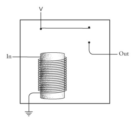
When an incoming current triggers the electromagnet, the electromagnet pulls down a flexible strip of metal that acts like a switch to turn on an outgoing current:
