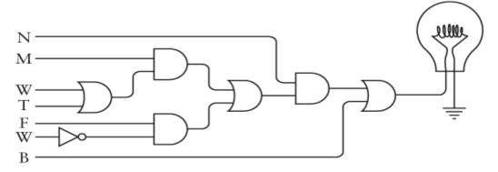
The symbols down the left side of the circuit diagram are in the same order as they appear in the expression. These signals come from the switches wired with inverters and the 2-line-to-4-line decoder. Notice the use of the inverter for the (1 - W) part of the expression.
