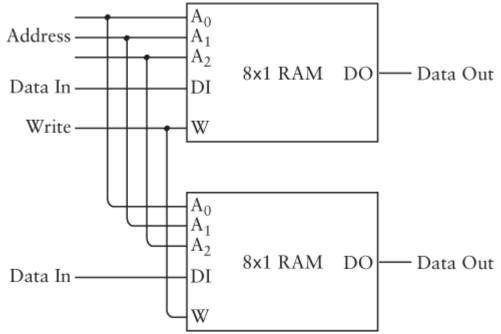
The Address and Write inputs of the two 8 x 1 RAM arrays are connected, so the result is an 8 x 2 RAM array:
