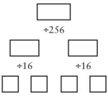
Start at the top. With each division, the quotient goes in the box to the left below the divisor, and the remainder goes in the box to the right. For example, here's the conversion of 51,966:
