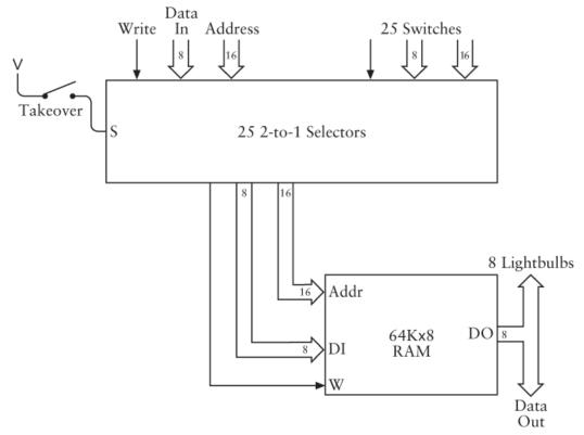
When the Takeover switch is open (as shown), the Address, Data input, and Write inputs to the 64K x 8 RAM array come from external signals shown at the top left of the 2-to-1 Selectors. When the Takeover switch is closed, the Address, Data input, and Write signals to the RAM array come from the switches on the control panel. In
