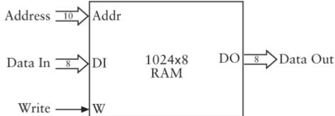
This RAM array stores a total of 8196 bits, organized as 1024 values of eight bits each. There are ten Address inputs because 2<sup>10</sup> equals 1024. There are eight Data inputs and eight Data outputs.
