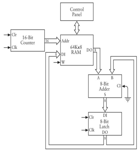
I've eliminated some other parts of the automated adder in this diagram as well, specifically the oscillator and the Clear switch. I removed them because it's no longer at all obvious where the Clear and Clock inputs to the counter and the latch will come from. Moreover, now that we've made use of the RAM data inputs, we need a way to control the RAM Write signal.
