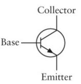
A small voltage on the base can control a much larger voltage passing from the collector to the emitter. If there's no voltage on the base, it effectively turns off the transistor.
