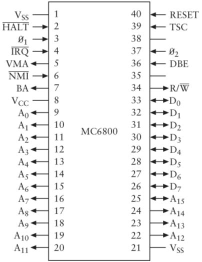
The V<sub>ss</sub> indicates Ground, and V<sub>cc</sub> is 5 volts. Like the 8080, the 6800 has 16 output Address signals and 8 Data signals used for both input and output. There's a RESET signal and a  $R/\overline{W}$  (read/write) signal. The  $\overline{IRQ}$  signal stands for *interrupt request*. The signal timing of the 6800 is considered to be much simpler than that of the 8080.
