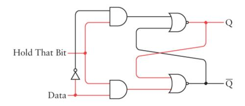
The Q output is now the same as the Data input, and  $\overline{Q}$  is the opposite. Now Hold That Bit can go back to being 0:
