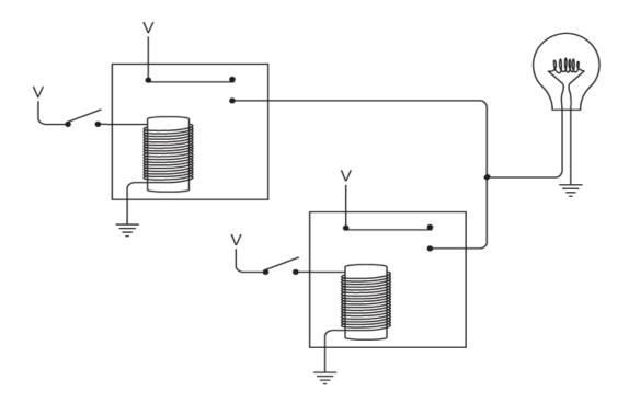
Notice that the outputs of the two relays are connected to each other. This connected output then provides power for the lightbulb. Either one of the two relays is enough to light the bulb. For example, if we close the top switch, the bulb lights up. The bulb is getting power from the left relay.
