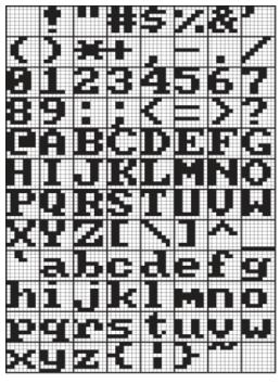
These are the characters corresponding to ASCII codes 20h through 7Fh. (No visible characters are associated with ASCII codes 00h through 1Fh.)
