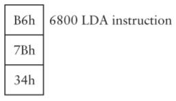
This sequence of bytes loads accumulator A with the byte stored at memory address 7B34h.
