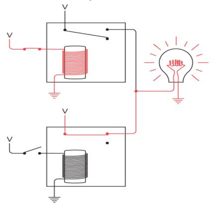
Similarly, the lightbulb remains on when the bottom switch is closed:
