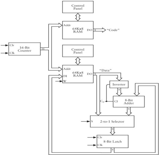
Now suppose we wish to add 56h and 2Ah together and then subtract 38h from the sum. You can do it with the following codes and data stored in the two RAM arrays:
