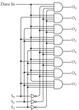
Again, notice that the inputs to the sixth AND gate from the top include  $S_0$ ,  $\overline{S}_1$ ,  $S_2$ . No
