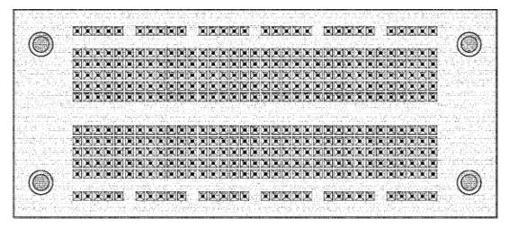
Each short row of 5 holes is electrically connected underneath the plastic base. You insert chips into the breadboard so that a chip straddles the long central groove and the pins go into the holes on either side of the groove. Each pin of the IC is then electrically connected to 4 other holes. You connect the chips with pieces of wires pushed into the other holes.
