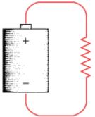
The squiggly line is recognizable to electrical engineers as the symbol for a resistor. Here it means that the circuit has a resistance that is neither very low nor very high.
