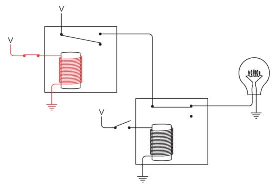
The light goes off because power is no longer being supplied to the second relay. Similarly, if the bottom switch is closed, the light is also off:
