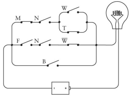
Although the M, T, and NOT W switches are closed, we don't have a complete circuit to light up the lightbulb. Next the salesperson brought out a neutered white female:
