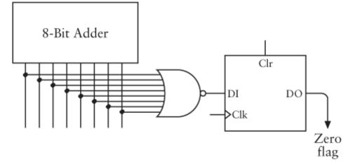
The output of that 8-bit NOR gate is 1 only if all the inputs are 0. Like the Clock input of the Carry latch, the Clock input of the Zero latch latches a value only when an *Add*, *Subtract, Add with Carry*, or *Subtract with Borrow* instruction is being performed. This latched value is known as the *Zero flag*. Watch out because it could seem as if it's working backward: The Zero flag is 1 if the output of the adder is all zeros, and the Zero flag is 0 if output of the adder is not all zeros.
