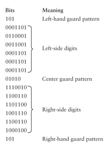
The first 3 bits are always 101. This is known as the *left-hand guard pattern*, and it allows the computer-scanning device to get oriented. From the guard pattern, the scanner can determine the width of the bars and gaps that correspond to single bits. Otherwise, the UPC would have to be a specific size on all packages.
