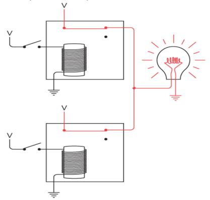
In this case, the two outputs are connected, which is similar to the OR configuration but using the other contacts. The lightbulb is on when both switches are open.
