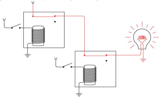
If the top switch is closed, the bulb goes off:
