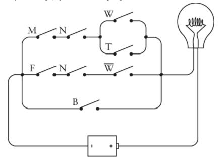
Each switch in this circuit is labeled with a letter—the same letters as in the Boolean expression. ( $\overline{W}$  means NOT W and is an alternative way to write 1 – W). Indeed, if
