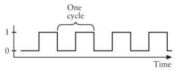
The time required for one cycle is called the *period* of the oscillator. Let's assume that we're looking at a particular oscillator that has a period of 0.05 second. We can then label the horizontal axis in seconds beginning from some arbitrary time we denote as 0:
