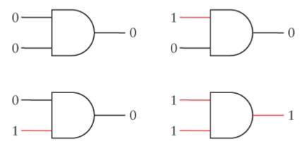
As with the two switches wired in series, the AND gate can also be described in this little table:
