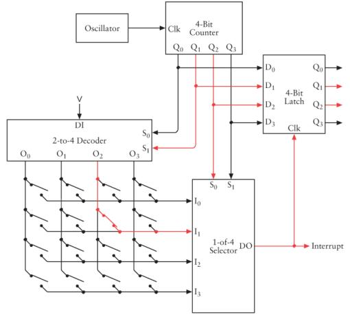
That's the code corresponding to that key. When that key is pressed, no other counter output will cause the output of the selector to be 1. Each key has its own code.
