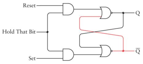
Recall that the output of an AND gate is 1 only if both inputs are 1. In this diagram, the Q output is 0 and the  $\overline{Q}$  output is 1.
