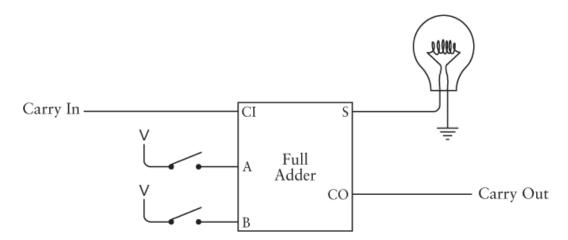
The carry output from the first Full Adder is an input to this second Full Adder. Each subsequent column of digits is wired the same way. Each carry output from one column is a carry input to the next column.
