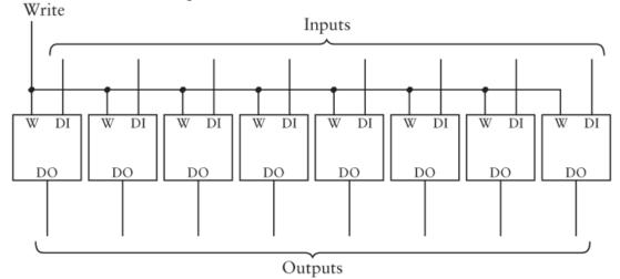
This 8-bit latch has eight inputs and eight outputs. In addition, the latch has a single input named Write that's normally 0. To save an 8-bit value in this latch, make the Write input 1 and then 0 again. This latch can also be drawn as a single box, like so:
