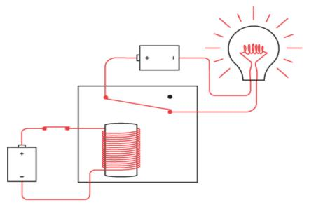
When the electromagnet pulls the metal contact, the relay is said to be *triggered*. When the switch is turned off, the iron bar stops being magnetic, and the metal contact returns to its normal position.
