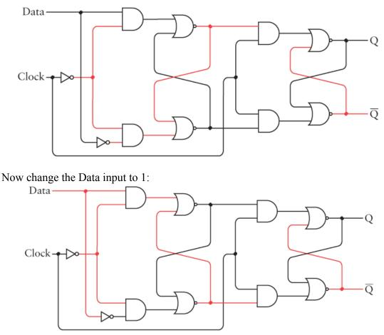
This changes the first flip-flop stage because the inverted Clock input is 1. But the second stage remains unchanged because the uninverted Clock input is 0. Now change the Clock input to 1:
