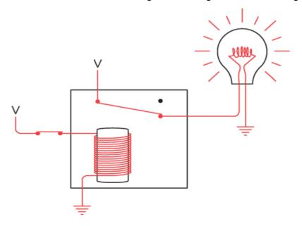
These diagrams of the relay show two voltage sources and two grounds, but in all the diagrams in this chapter, all the V's can be connected to one another and all the grounds can be connected to one another. All the networks of relays and logic gates in this chapter and the next will require only one battery, although it might need to be a big battery. For example, the preceding diagram can be redrawn with only one battery like this:
