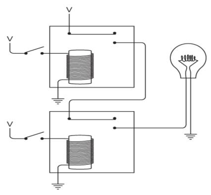
The output of the top relay supplies a voltage to the second relay. As you can see, when both switches are open, the lightbulb isn't lit. We can try closing the top switch:
