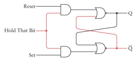
It behaves like a normal R-S flip-flop because now the output of the upper AND gate is the same as the Reset signal, and the output of the lower AND gate is the same as the Set signal.
