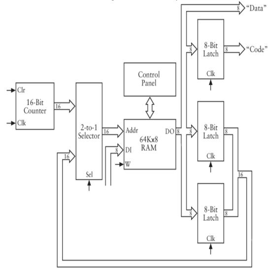
We've made a lot of progress. Now it's possible to enter the instructions and the data in a single RAM array. For example, the diagram on the next page shows how to add two 8-bit numbers together and subtract a third.
