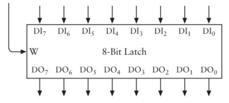
Or to be more consistent with the 1-bit latch, it can be drawn this way:
