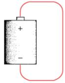
This is known as a *short circuit*. The voltage is still 1.5, but the resistance is now very, very low. The current is 1.5 volts divided by a very small number. This means that the current will be very, very high. Lots and lots of electrons will be flowing through the wire. In reality, the actual current will be limited by the physical size of the battery.
