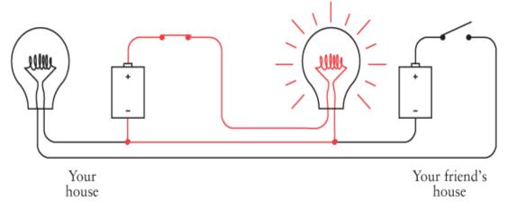
No electricity flows in the other part of the circuit because there's no place for the electrons to go to complete a circuit.
