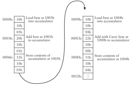
At the completion of these six instructions, the 16-bit value at memory locations 1004h and 1005h will equal A7h times 1. Therefore, these six instructions have to be repeated 27 more times in order for that 16-bit value to equal A7h times 1Ch. You can achieve this by typing in these six instructions 27 more times beginning at address 0012h. Or you can put a *Halt* instruction at 0012h and press the Reset button 28 times to get the final answer.
