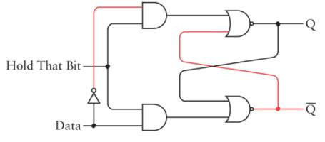
In this case, both inputs are 0 and the output Q is 0 (which means that  $\overline{Q}$  is 1). As long as Hold That Bit is 0, the Data input has no effect on the circuit:
