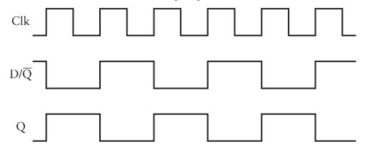
When the Clock input goes from 0 to 1, the value of D (which is the same as  $\overline{\mathbb{Q}}$ ) is
