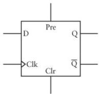
You'll recall that the Preset and Clear inputs should both be 0 for normal operation. But if Preset is 1, Q becomes 1. And if Clear is 1, Q becomes 0.
