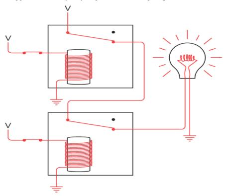
Now both relays are triggered, and current can flow between V, the lightbulb, and ground.
