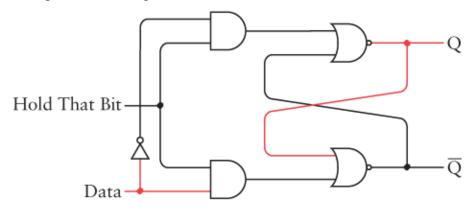
The circuit now remembers the value of Data when Hold That Bit was last 1, regardless of how Data changes. The Data signal could, for example, go back to 0 with no effect on the output:
