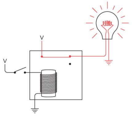
In this case, the lightbulb goes out when you close the switch. A single relay wired in this way is called an *inverter*. An inverter isn't a logic gate (logic gates always have two or more inputs), but it's often very useful nonetheless. It's represented by a special symbol that looks like this:
