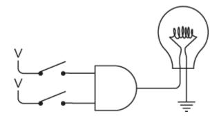
Notice that this symbol for the AND gate not only takes the place of two relays wired in series, but it also implies that the top relay is connected to a voltage, and both relays are connected to ground. Again, the lightbulb lights up only if both the top switch *and* the bottom switch are closed. That's why it's called an *AND gate*.
