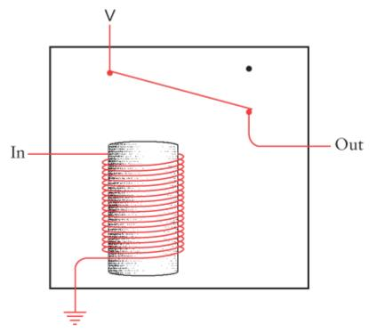
So a telegraph key, a relay, and a sounder are connected more or less like this:
