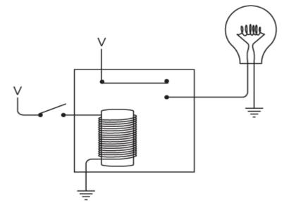
When the switch is closed, a current flows between V and ground through the coils of the electromagnet. This causes the electromagnet to pull the flexible metal contact. That connects the circuit between V, the lightbulb, and ground. The bulb lights up:
