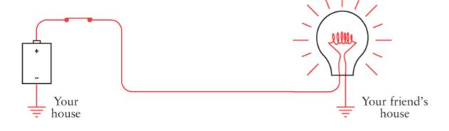
The electrons come out of the earth at your friend's house, go through the lightbulb and wire, the switch at your house, and then go into the positive terminal of the battery. Electrons from the negative terminal of the battery go into the earth.
