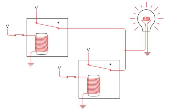
What we have here is a situation in which the bulb lights up if the top switch *or* the bottom switch is closed. The key word here is *or*, so this is called the *OR gate*. Electrical engineers use a symbol for the OR gate that looks like this:
