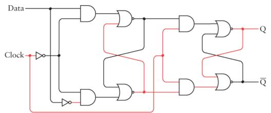
The Q and  $\overline{Q}$  outputs can change only at the instant that the Clock input changes from 0 to 1.
