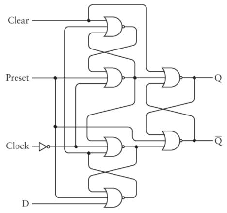
The Preset and Clear inputs override the Clock and Data inputs. Normally these two inputs are 0. When the Preset input is 1, Q becomes 1 and  $\overline{Q}$  becomes 0. When the Clear input is 1, Q becomes 0 and  $\overline{Q}$  becomes 1. (Like the Set and Reset inputs of an R-S flip-flop, Preset and Clear shouldn't be 1 at the same time.) Otherwise, this behaves like a normal edge-triggered D-type flip-flop:
