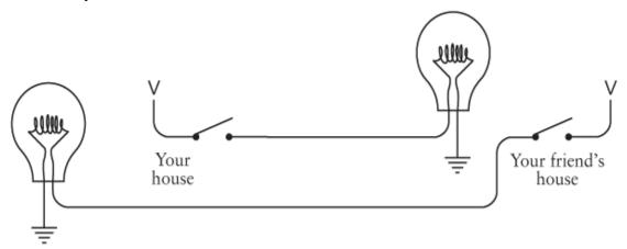
This circuit is functionally the same as the configuration shown previously, in which three wires crossed the fence between the houses.
