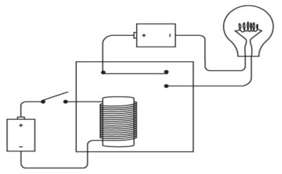
Notice that the switch at the left is open and the lightbulb is off. When you close the switch, the battery at the left causes current to flow through the many turns of wire around the iron bar. The iron bar becomes magnetic and pulls down a flexible metal contact that connects the circuit to turn on the lightbulb:
