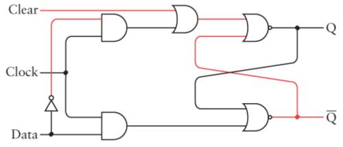
This signal forces Q to be 0 regardless of the other input signals, in effect clearing the flip-flop.
