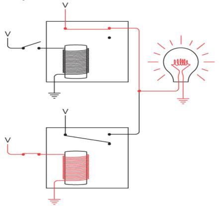
Only when both switches are closed does the lightbulb go off:
