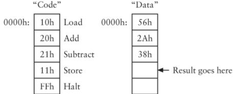
After the *Load* operation, the accumulator contains the value 56h. After the *Add* operation, the accumulator contains the sum of 56h and 2Ah, or 80h. The *Subtract* operation causes the bits of the next value in the Data RAM array (38h) to be inverted. The inverted value C7h is added to 80h with the carry input of the adder set to 1:
