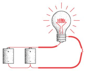
This works. The batteries are said to be connected *in parallel* rather than *in series* as shown earlier. The combined voltage is 1.5 volts, which is the same as the voltage of each of the batteries. The light will probably still glow, but not as brightly as with two batteries in series. But the batteries will last twice as long.
