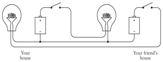
Notice that the negative terminals of the two batteries are now connected. The two circular circuits (battery to switch to bulb to battery) still operate independently, even though they're now joined like Siamese twins.
