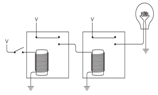
When you turn the switch on, the first relay is triggered, which then provides a voltage to the second relay. The second relay is triggered and the light goes on:
