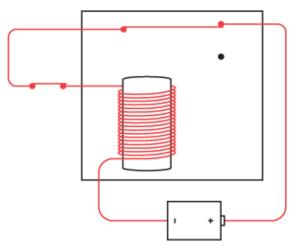
The completed circuit causes the electromagnet to pull down the flexible contact:
