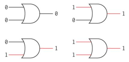
In the same way that we summarized the output of the AND gate, we can summarize the output of the OR gate:
