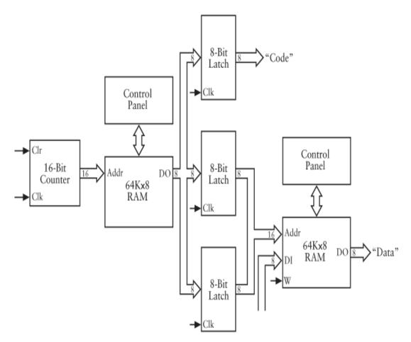
The process of retrieving an instruction from memory is known as the *instruction fetch*. In our machine, each instruction is 3 bytes in length, and it's retrieved from memory 1 byte at a time; the instruction fetch requires three cycles of the Clock signal. The entire *instruction cycle* requires a fourth cycle of the Clock signal. These changes certainly complicate the control signals.
