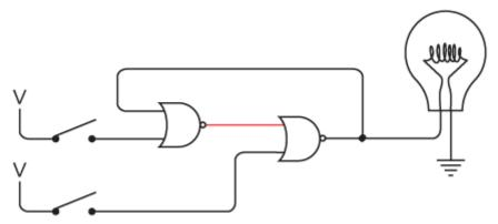
Notice the oddly contorted wiring: The output of the NOR gate on the left is an input to the NOR gate on the right, and the output of the right NOR gate is an input to the left NOR gate. This is a type of *feedback*. Indeed, just as in the oscillator, an output circles back to become an input. This idiosyncrasy will be a characteristic of most of the circuits in this chapter.
