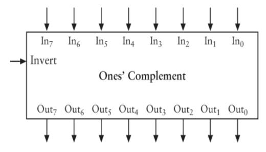
The Ones' Complement box, the 8-Bit Adder box, and a final exclusive OR gate can now be wired together like this:
