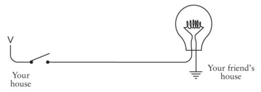
The V stands for *voltage*, but it could also stand for *vacuum*. Think of the V as an electron vacuum and think of the ground as an ocean of electrons. The electron
