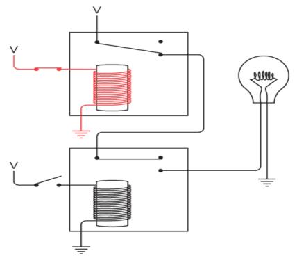
Still the lightbulb doesn't light because the bottom switch is still open and that relay isn't triggered. We can try opening the top switch and closing the bottom switch:
