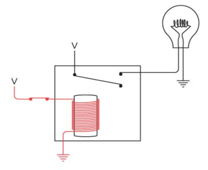
Using the terminology of switches, this type of relay is called a *double-throw* relay. It has two outputs that are electrically opposite—when one has a voltage, the other doesn't.
