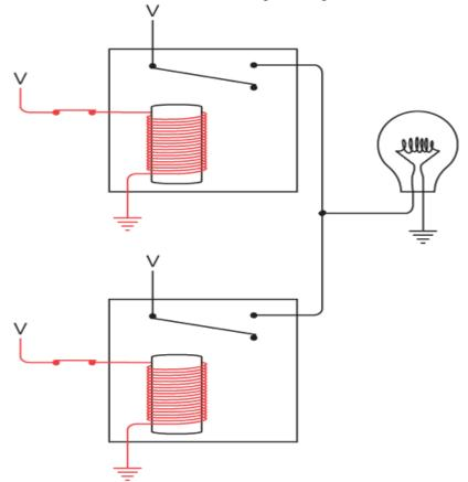
This behavior is exactly opposite that of the AND gate. This is called *NOT AND* or, more concisely, *NAND*. The NAND gate is drawn just like the AND gate but with a circle at the output, meaning the output is the inverse of the AND gate:
