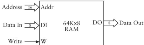
Why 64 KB? Why not 32 KB or 128 KB? *Because 65,536 is a nice round number*. It's 2<sup>16</sup>. This RAM array has a 16-bit address. In other words, the address is 2 bytes exactly. In hexadecimal, the address ranges from 0000h through FFFFh.
