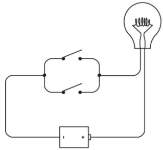
These switches are said to be connected *in parallel*. The difference between this and the preceding connection is that this lightbulb will light if you close the top switch:
