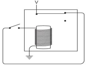
You might recognize in this diagram the inverter from Chapter 11. The circuit can be drawn more simply this way:
