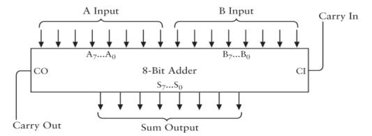
As you probably recall, the inputs A0 through A7 and B0 through B7 were connected to switches that indicated two 8-bit values to be added. The Carry In input was connected to ground. The S0 through S7 outputs were connected to eight lightbulbs that displayed the result of the addition. Because the addition could result in a 9-bit value, the Carry Out output was also connected to a ninth lightbulb.
