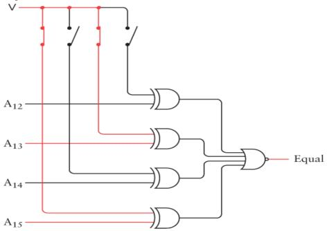
You can then combine that Equal signal with a 2-Line-to-4-Line Decoder to generate
