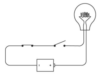
Similarly, if you leave the left switch open and close the right switch, nothing happens. The lightbulb lights up only if both the left switch and the right switch are closed, as shown on the next page.
