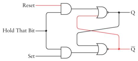
Only when the Hold That Bit signal is 1 will this circuit function the same way as the normal R-S flip-flop shown earlier:
